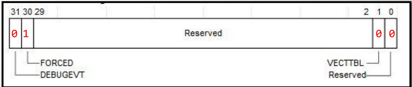
When this bit is set to 1, the HardFault handler must read the other fault status registers to find the cause of the fault.
